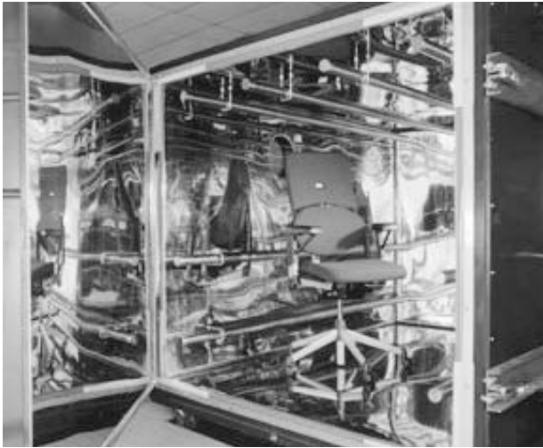
An office chair in an environmental testing chamber is being prepared for emissions testing for compliance with the GREENGUARD Certification Standard for Chemical Emissions. Image courtesy of Air Quality Sciences Inc.
