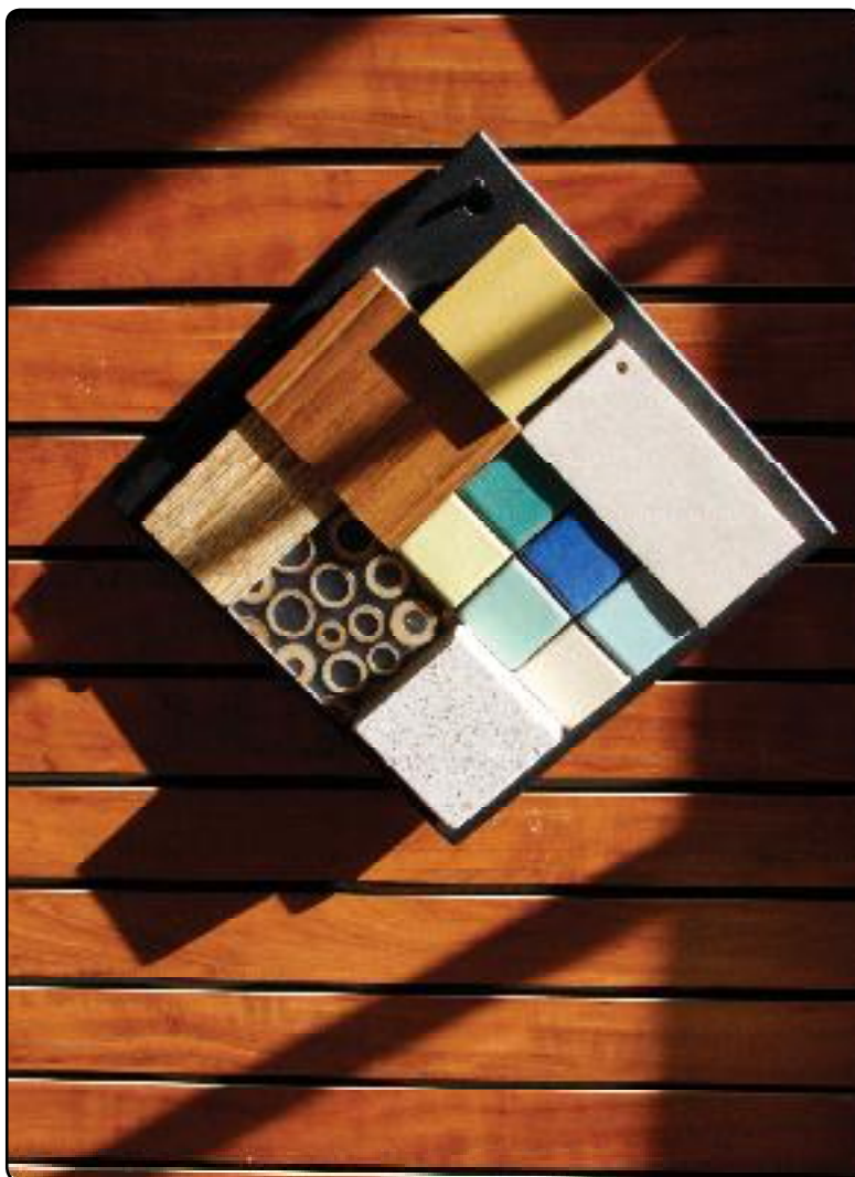
Clockwise, from top: Paperstone, marmoleum, recycled tile, lcestone, eco-resin, kirei and bamboo. These green and recycled products, and more, are available at Build It Naturally in downtown Asheville. photo by Jonathan Welch
