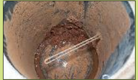
Electric Storage Water Heater After 90 Days Using Unsoftened Water
