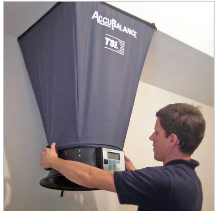
Diagnostic airflow testing being performed at a final Green Built NC inspection for quality assurance. Home Energy Partners photo
