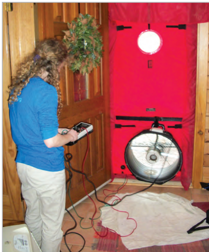
Green certifications require performance testing, such as the iconic blower-door test of house air-tightness. Knowing a house is going to be tested — and must pass the test — makes everyone involved in building it likely to be more thorough with the details. STEVE LINTON PHOTO
