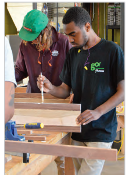
YouthBuild students Atticus Monfredi (left) and Erik Whitesides practice clamping and gluing hardwoods to create cutting boards for GO's culinary training program graduates.
