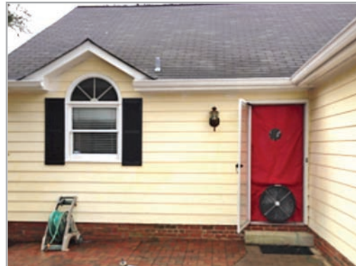
Above: Holes in the ceiling can waste a lot of energy. Here interior walls are drawing in hot attic air. Attic air sealing will stop this. Below, left: A blower door is set up for a Green Gauge assessment. Air leakage will be tested. Below, right: Interior wall top plates and plumbing holes as seen from the attic. These gaps allow a lot of air to escape or enter the home. Kevin Bauguss photos
